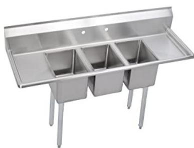
Dishwashers are **optional** but a 3-compartment sink is **required** in a facility using multi-use kitchenware items. Each compartment of this sink must be large enough to submerge at least half of the largest piece of equipment you have (e.g. - a small bar sink would be not acceptable for washing large pots, pans, and sheet trays).
